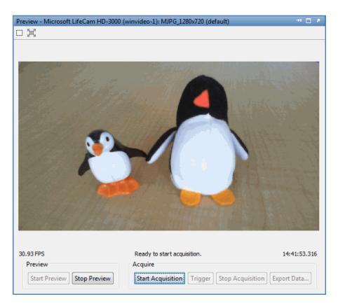
In the example shown here, the **Preview** panel of the Image Acquisition Tool is showing that frames are being acquired at an average of 30.93 FPS. The **Preview** panel also displays device, resolution, acquisition status, and the timestamp. The toolbox stand-alone **Preview** window shows those properties as well.
